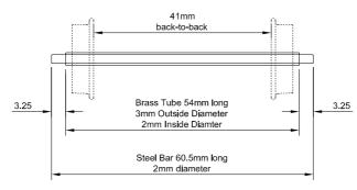
Wheels are friction-fit onto 3mm tube Glue axle bar inside tube with epoxy resin
